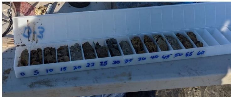
Photograph 4. Chip Tray Used to Collect 5-foot Samples for Lithologic Record
