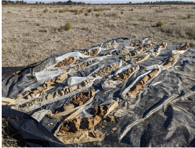
Photograph 3. Continuous Core Samples Collected During Drilling
