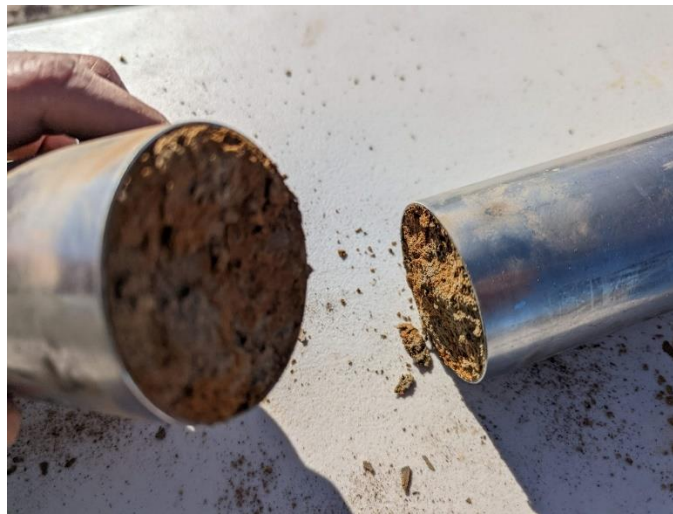
Photograph 5. Stainless Steel Rings Used for Collection of Drive Samples
