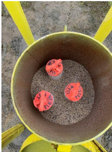
Photograph 8. Three Well Casing Within Well MW-1
