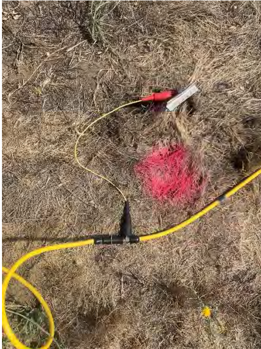
Photographs ERP lines with stainless steel electrode spikes. Profile lines used up to 56 spikes inserted into the ground at 15-foot intervals.
