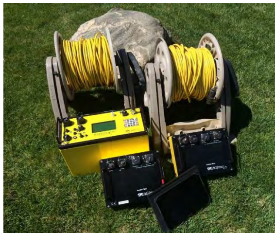
Figure 3: SuperSting R8 (yellow box), two 56-electrode switch boxes (black), WiFi tablet (foreground) and two communication cables on reels.
