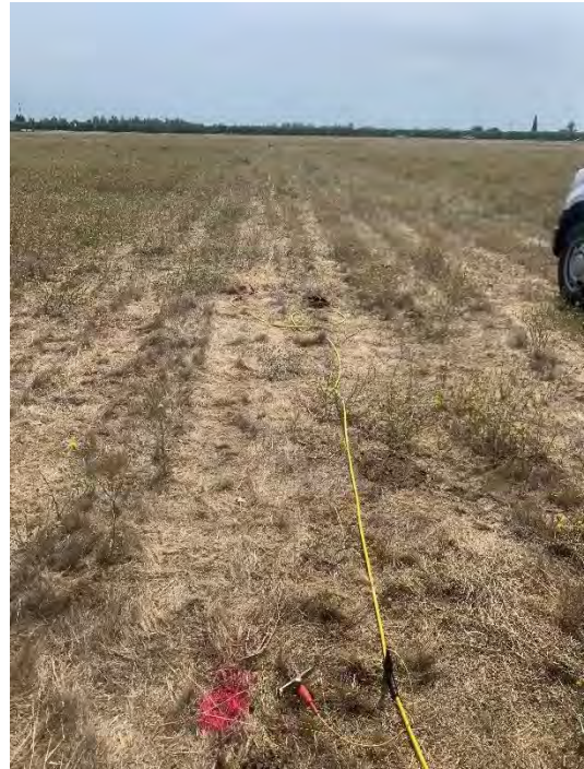
Photographs ERP lines with stainless steel electrode spikes. Profile lines used up to 56 spikes inserted into the ground at 15-foot intervals.
